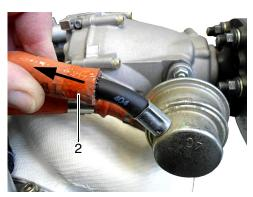
Pinch rubber hose to prevent fuel leakage:
