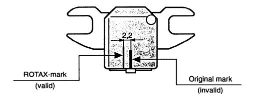
At an ignition timing check the supplementary mark of the pick-up has to be in line with the mark on the flywheel.
