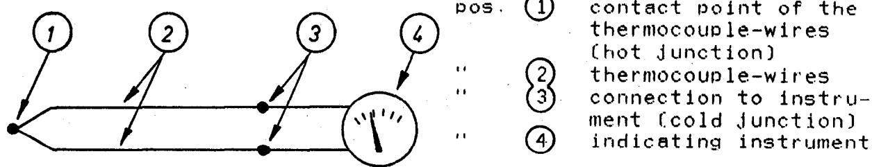
Depending on the temperature difference between hot and cold junction the thermocouple supplies the so-called thermo voltage indicated by the instrument which is calibrated in temperature degrees.
