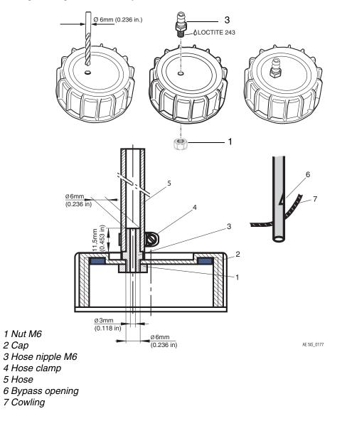
Fig. 1 Overflow bottle cap
